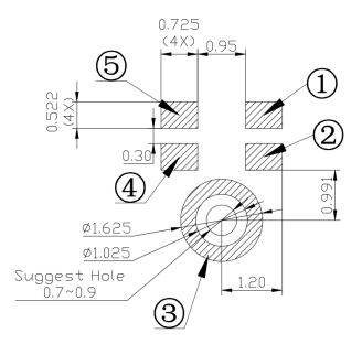
Figure 3. Recommended landing pattern on customers' PCB
