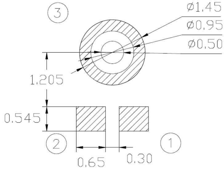
Figure 3. Recommended landing pattern on customers' PCB
