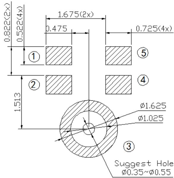
Figure 3. Recommended landing pattern on customers' PCB
