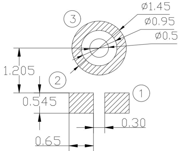
Figure 3. Recommended landing pattern on customers' PCB
