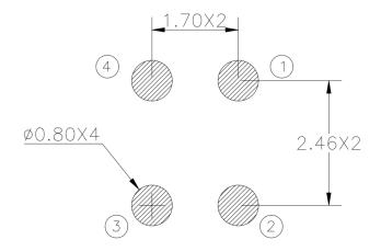
Figure 3. Recommended landing pattern on customers' PCB
